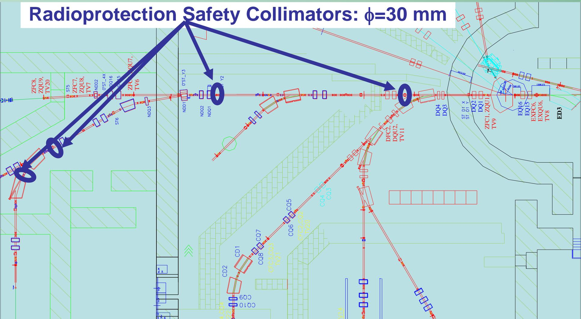
**We are replacing the radioprotection safety collimators using new faraday cups – this will give a larger transport efficiency with a further intensity gain from 2 to 4**
