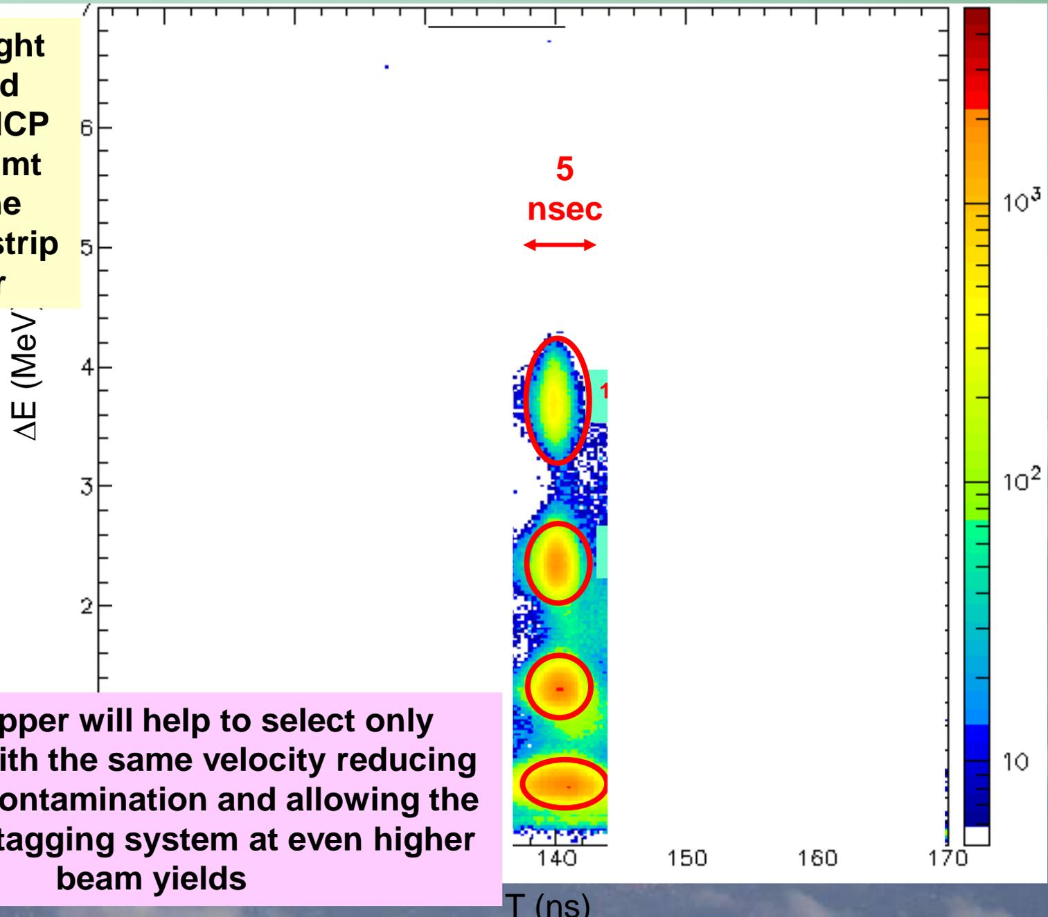
The chopper will help to select only particles with the same velocity reducing the beam contamination and allowing the use of the tagging system at even higher beam yields
