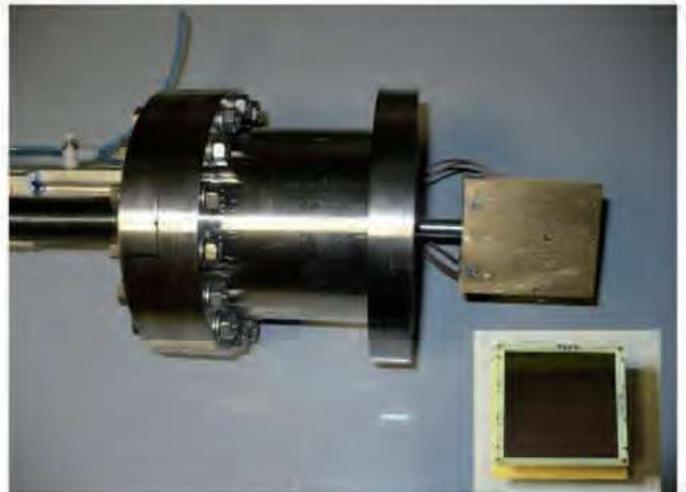
Fig. 3. PSD mounted in a pneumatic actuator. The mask made by brass is 2mm thick.
